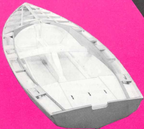
The Mark II Composite WAYFARER Stage II Hull
